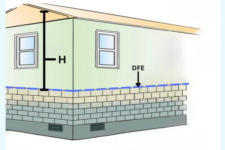
Design Flood Elevation (DFE) = Base Flood Elevation (BFE) + Freeboard
