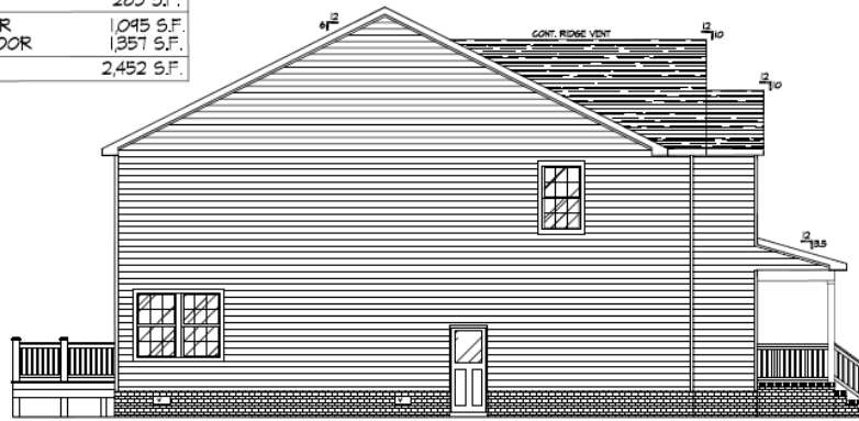
RIGHT SIDE ELEVATION SCALE: 1/4" = 1'-0"
