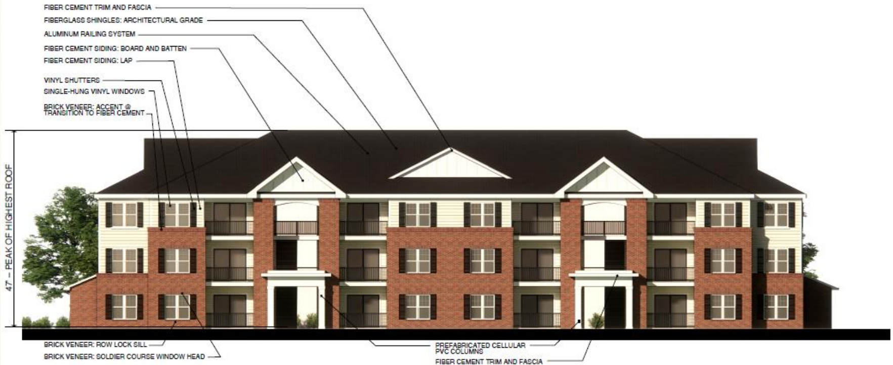
THREE-STORY BUILDINGS: ELEVATION AT ENTRANCE MATERIAL KEY
