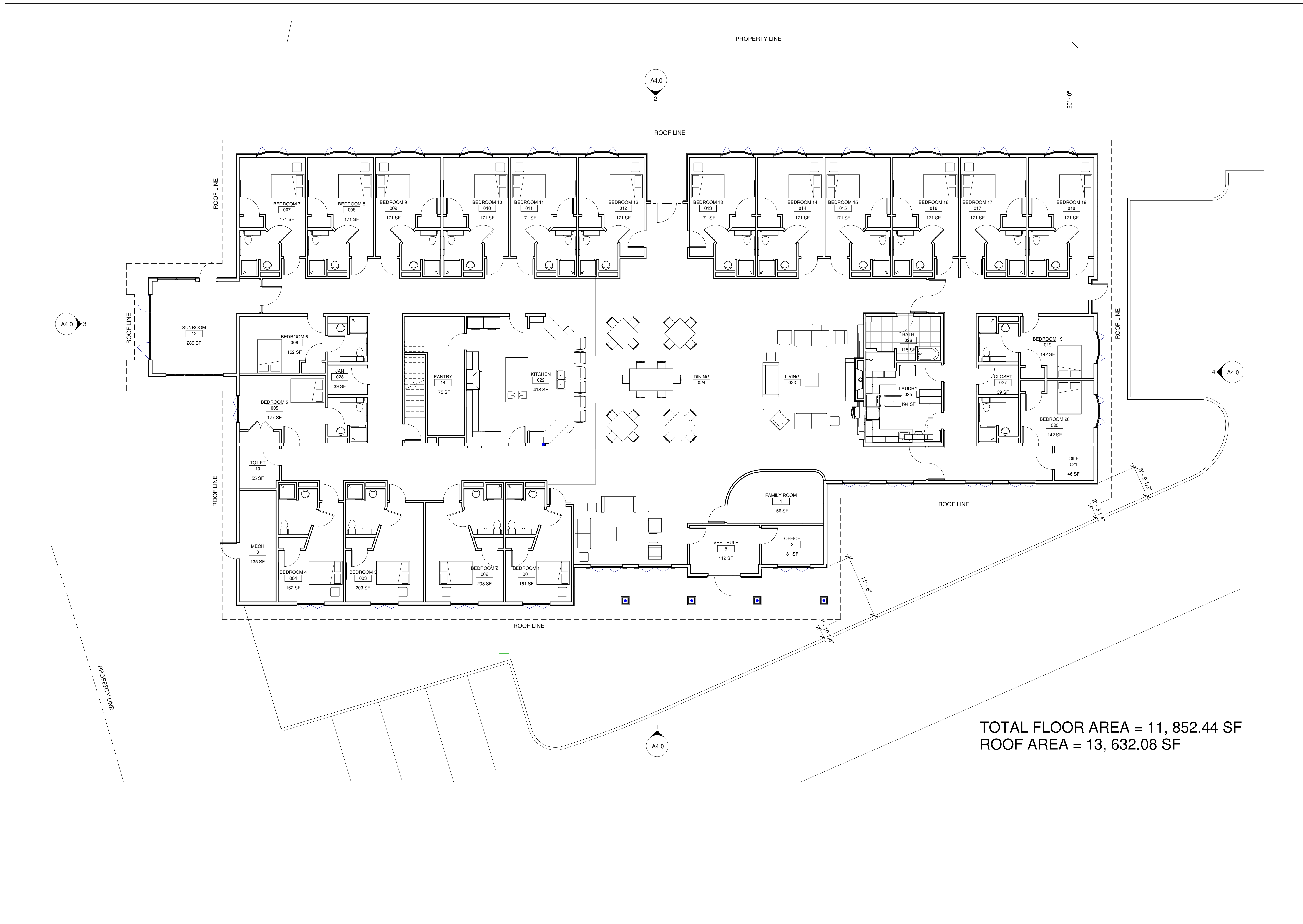
1 FLOOR PLAN A1.0 SCALE 1/8" = 1'-0"
