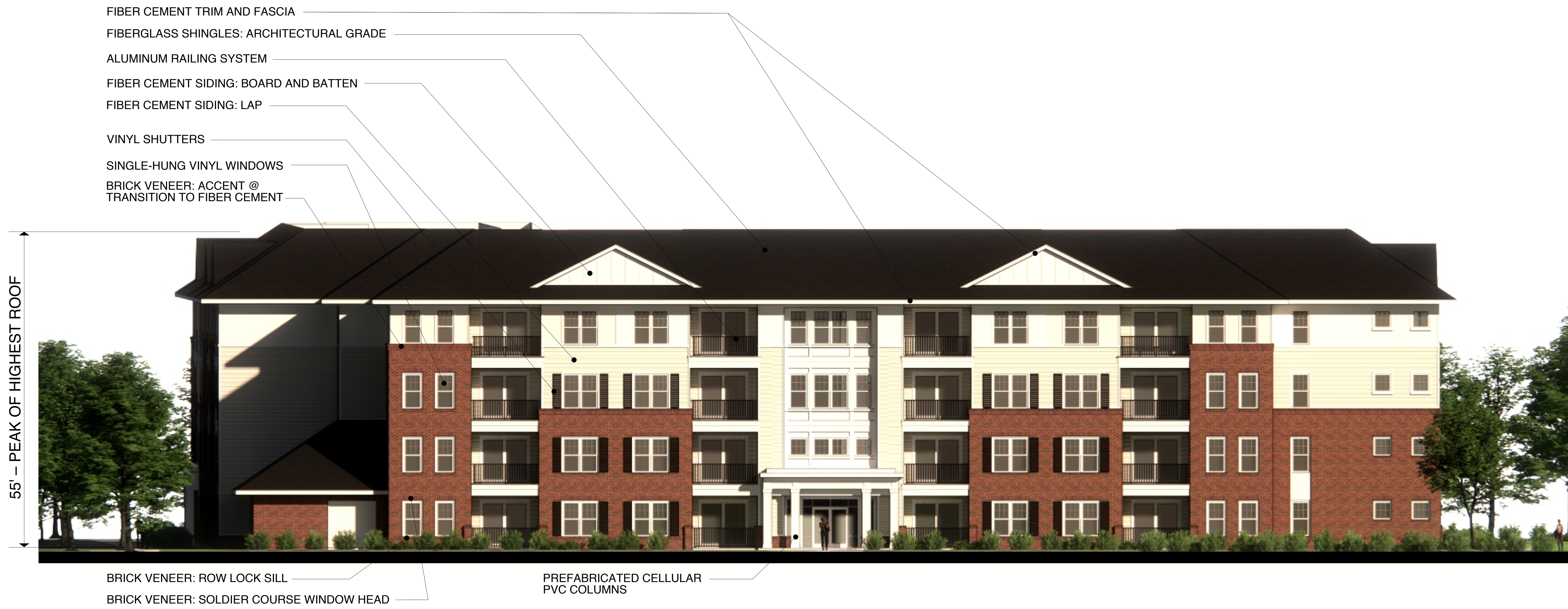
FOUR-STORY BUILDINGS: ELEVATION AT ENTRANCE MATERIAL KEY
