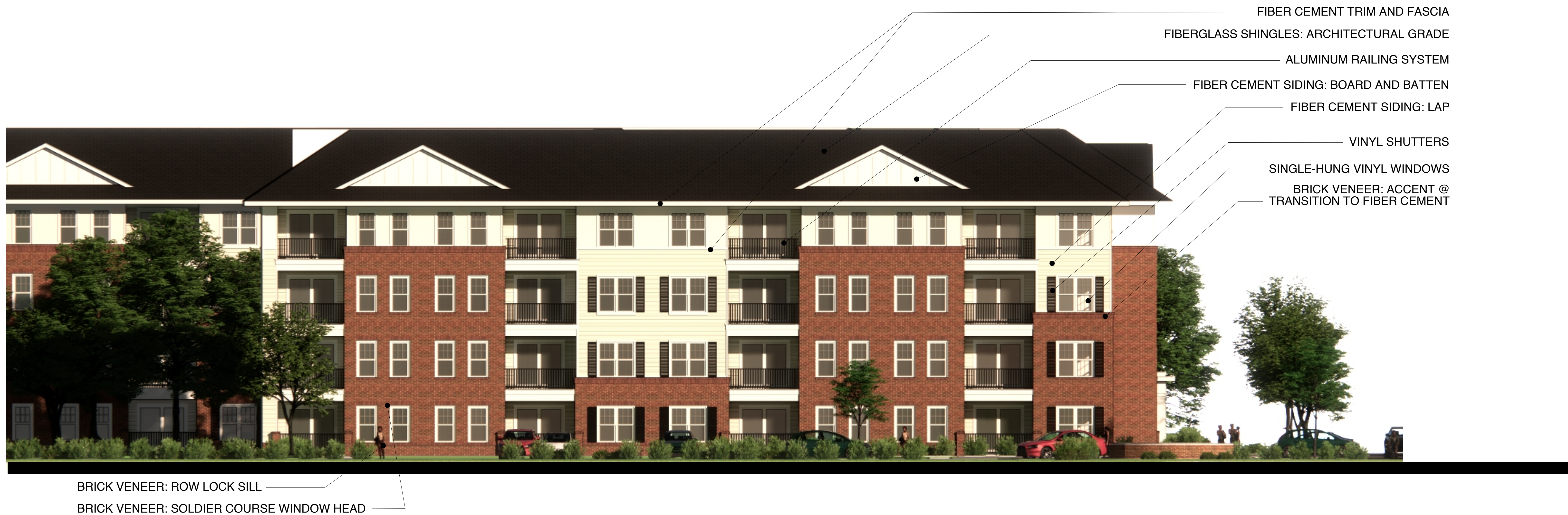
FOUR-STORY BUILDINGS: TYPICAL SIDE ELEVATION MATERIAL KEY
