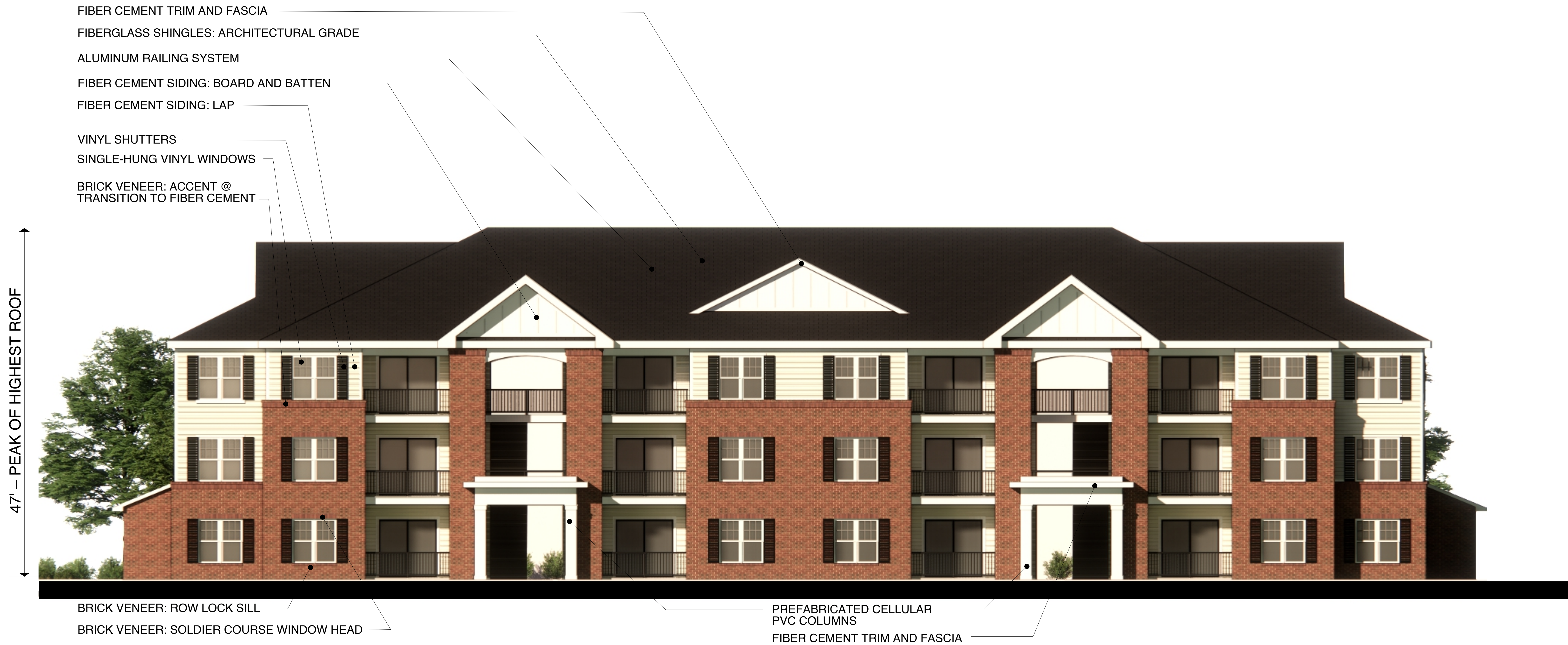
THREE-STORY BUILDINGS: ELEVATION AT ENTRANCE MATERIAL KEY
