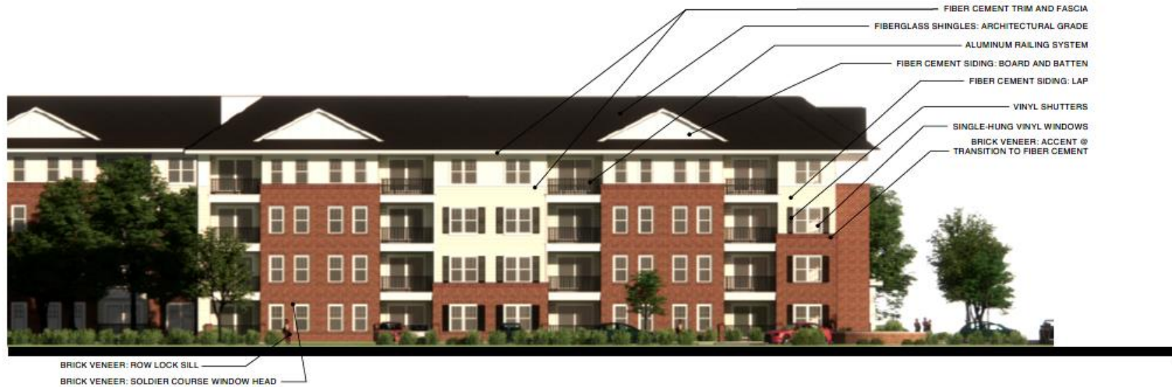
FOUR-STORY BUILDINGS: TYPICAL SIDE ELEVATION MATERIAL KEY
