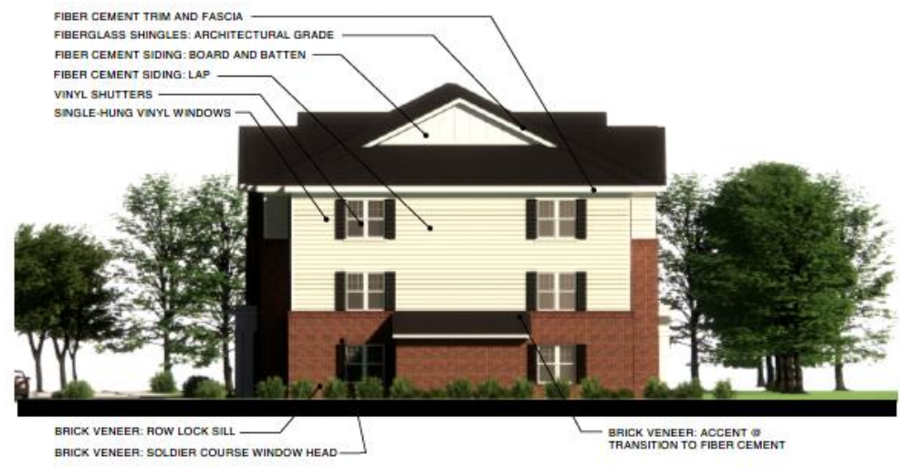
THREE-STORY BUILDINGS: ELEVATION AT END MATERIAL KEY
