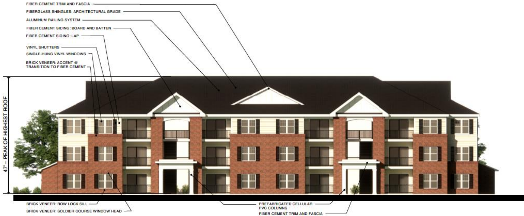
THREE-STORY BUILDINGS: ELEVATION AT ENTRANCE MATERIAL KEY
