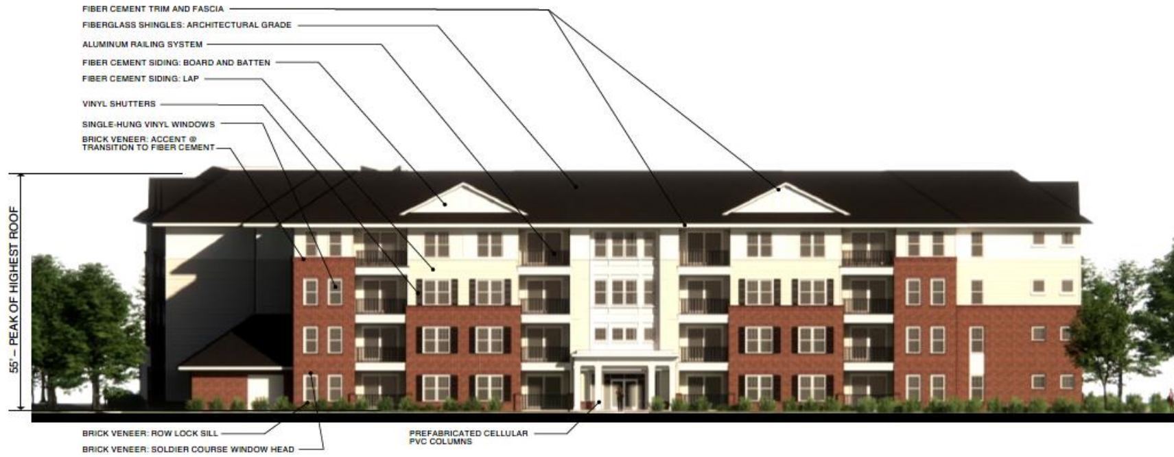
FOUR-STORY BUILDINGS: ELEVATION AT ENTRANCE MATERIAL KEY
