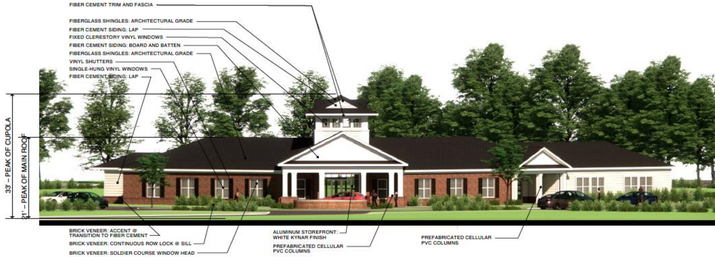
CLUBHOUSE: ELEVATION AT ENTRANCE MATERIAL KEY
