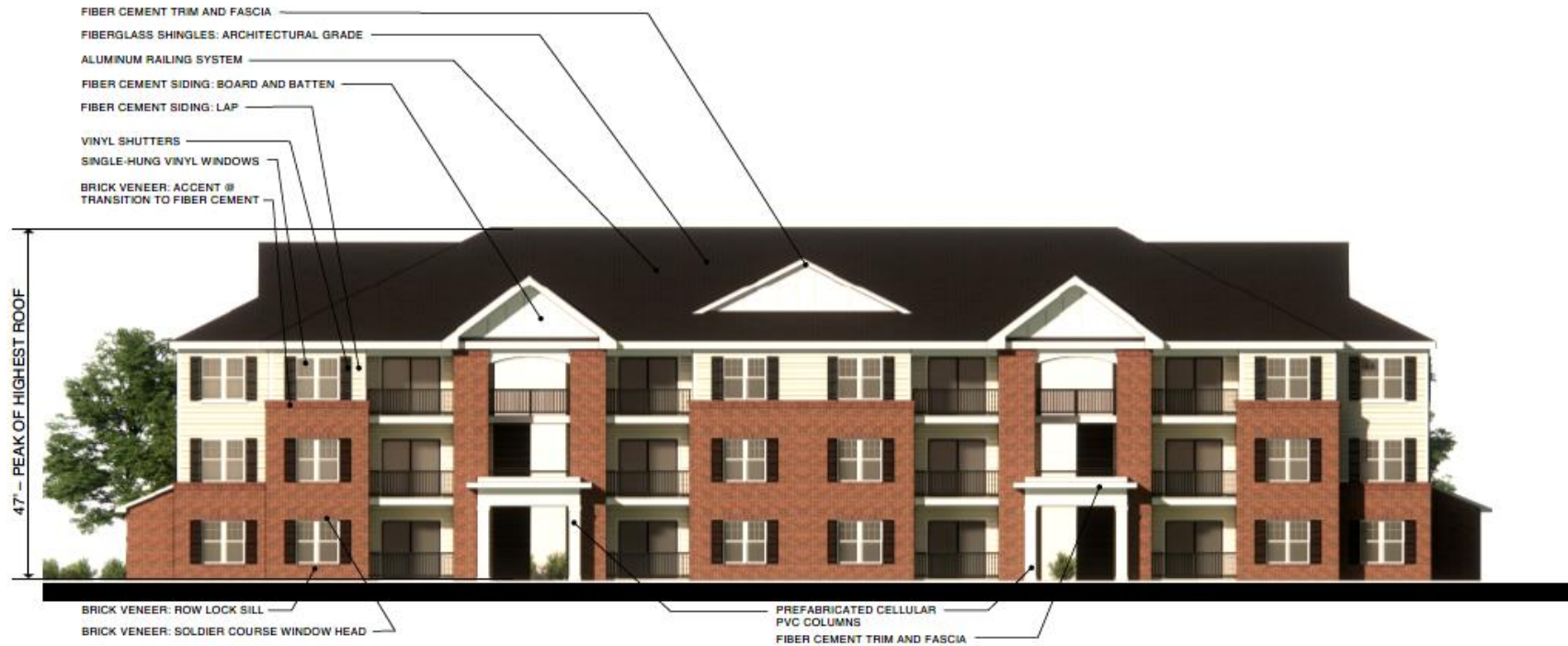
THREE-STORY BUILDINGS: ELEVATION AT ENTRANCE MATERIAL KEY
