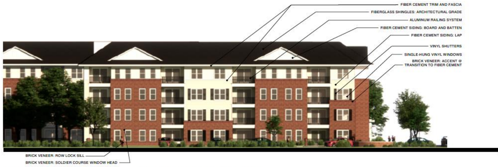
FOUR-STORY BUILDINGS: TYPICAL SIDE ELEVATION MATERIAL KEY
