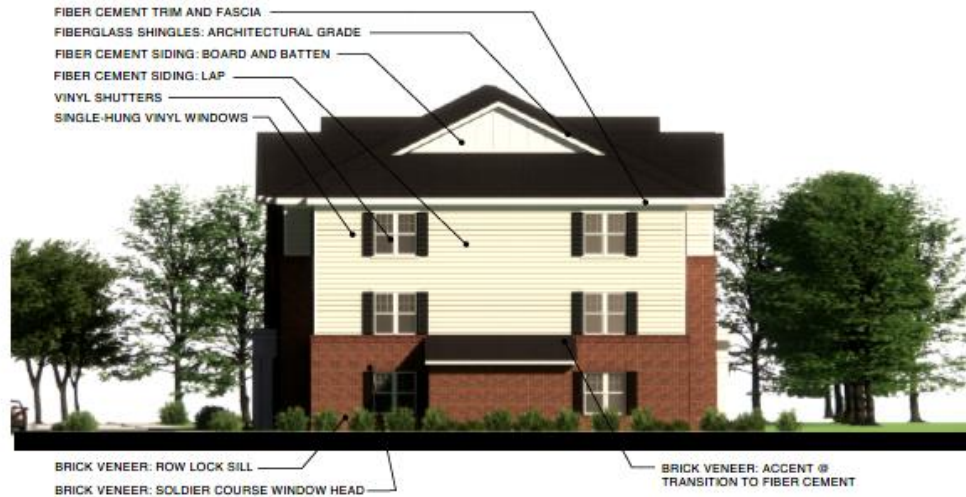
THREE-STORY BUILDINGS: ELEVATION AT END MATERIAL KEY
