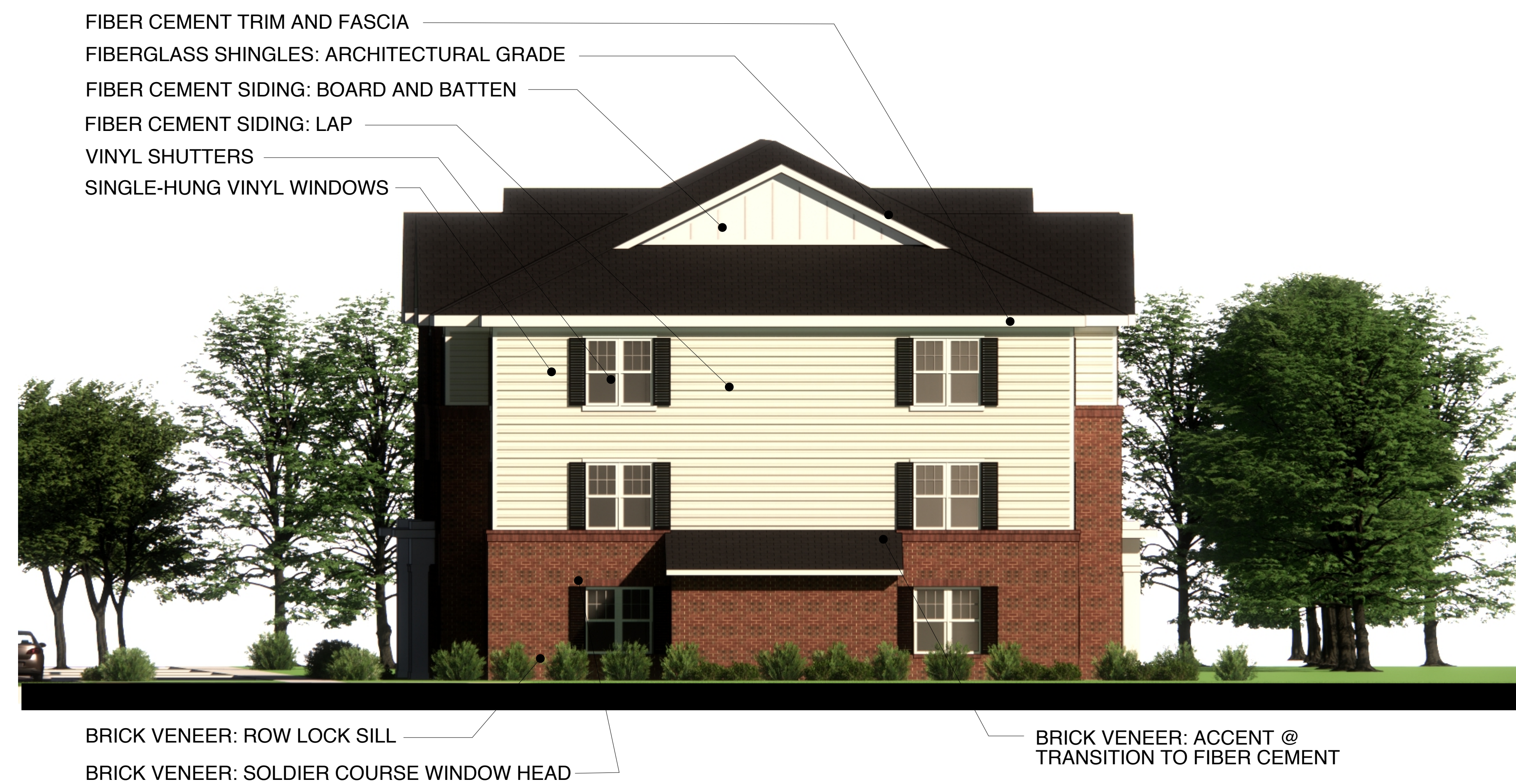
THREE-STORY BUILDINGS: ELEVATION AT END MATERIAL KEY
