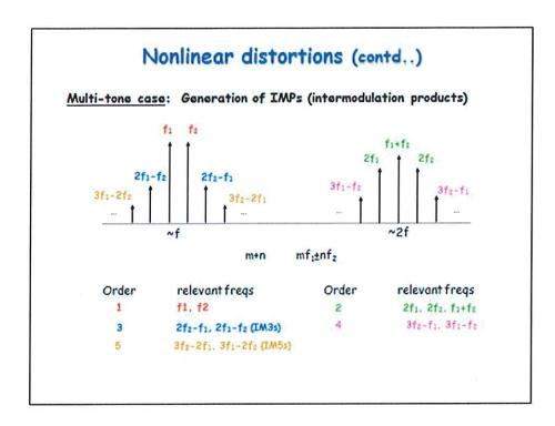
Not all of the mixing possibilities are significant in creating interference signals. Some fall "out-of-band" of the receiver and the higher order IM products are usually weaker in signal strength.
