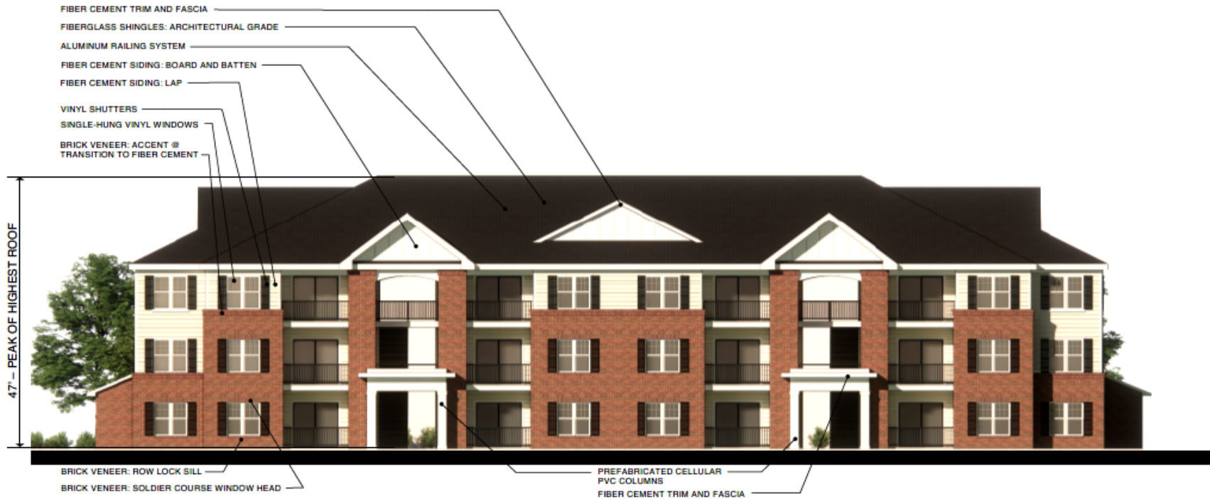
THREE-STORY BUILDINGS: ELEVATION AT ENTRANCE MATERIAL KEY
