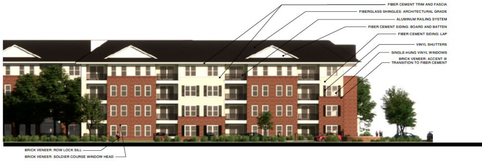
FOUR-STORY BUILDINGS: TYPICAL SIDE ELEVATION MATERIAL KEY
