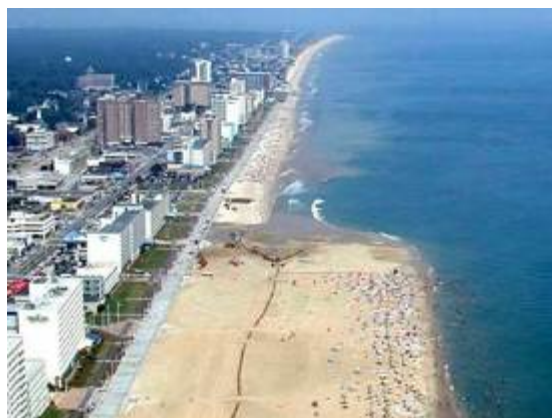
This photo, taken while the Virginia Beach Erosion Control and Hurricane Protection Project was underway, shows the significant difference between the unimproved area and the area of the widened beach berm already completed. (Source: City of Virginia Beach)
