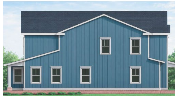
FRONT ELEVATION (BOARD & BATTEN) 1/4" = 1'-0"
