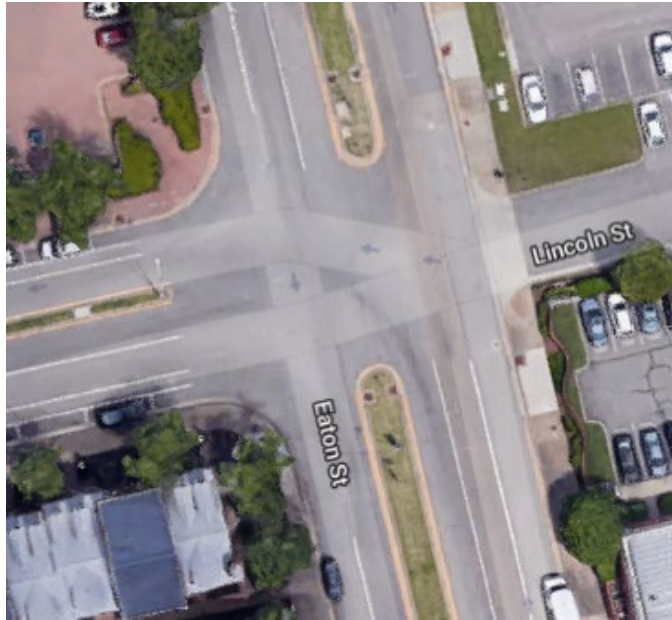
Eaton St & Lincoln St Crosswalks & Curb Bump Outs
