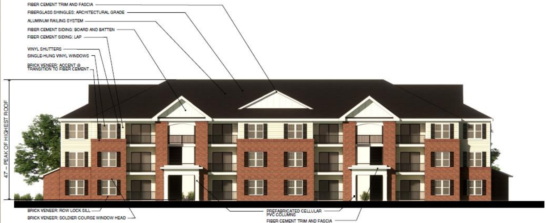
THREE-STORY BUILDINGS: ELEVATION AT ENTRANCE MATERIAL KEY
