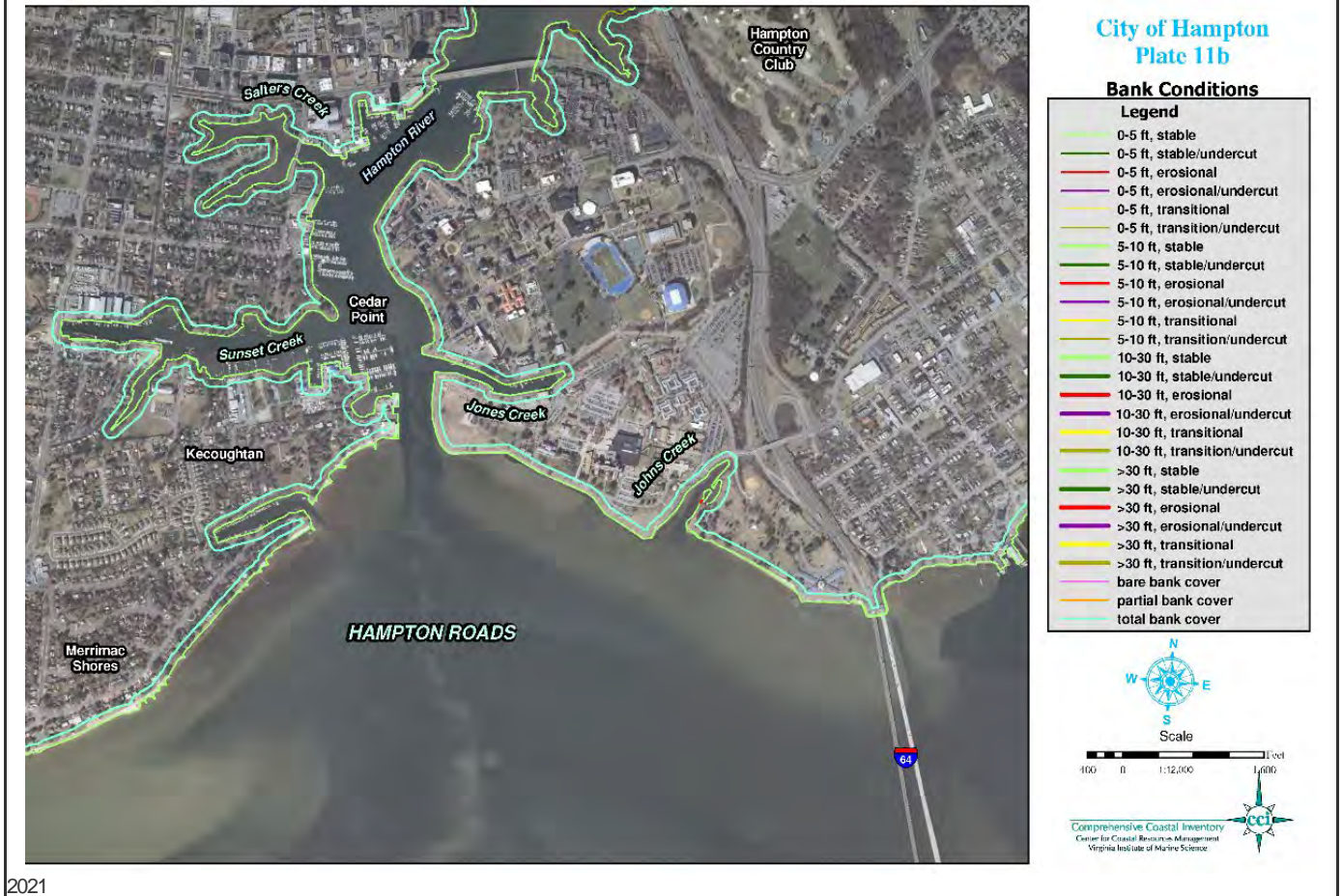
FIGURE 5.24: BANK CONDITIONS, HAMPTON RIVER
